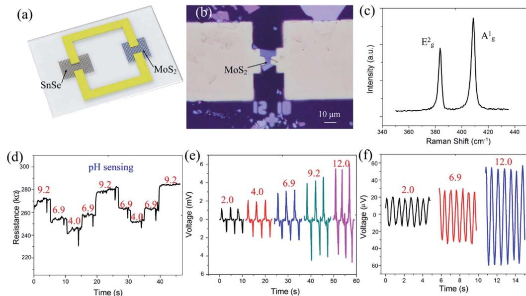
Fig. 5 (a) Schematic view of the SnSe nanogenerator integrated with a MoS<sub>2</sub> sensor. (b) Optical microscopy image of the MoS<sub>2</sub> sensor. (c) Raman spectrum of MoS<sub>2</sub>. (d) Dynamic resistance variation of the MoS<sub>2</sub> pH sensor as the pH value changes from 9.2 to 4.0. (e) The pH sensing performance of the SPSU upon periodic bending of the substrate. (f) The pH sensing performance of the SPSU by using heartbeats as the energy source.
