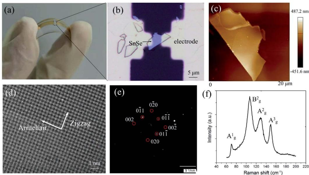
**Fig. 1** (a) Photo of the SnSe piezoelectric device. (b) Optical microscopy image of the SnSe piezoelectric device. (c) AFM topographic image of the SnSe flake. The SnSe flake is the same one demonstrated in (b). (d) High resolution TEM image of the SnSe crystal. (e) TEM diffraction image of SnSe. (f) Raman spectrum of SnSe.
